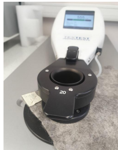
Fig.20 - Air permeability test
