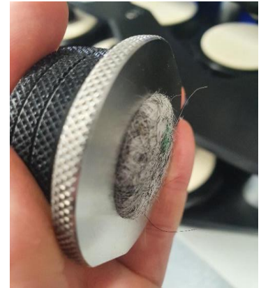
Fig.22 - Martindale abrasion test
